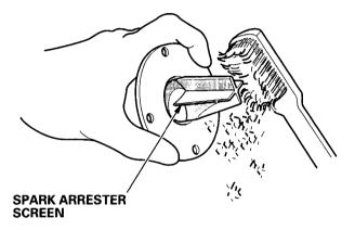
4. Install the spark arrester, and muffler protector in the reverse order of disassembly.
